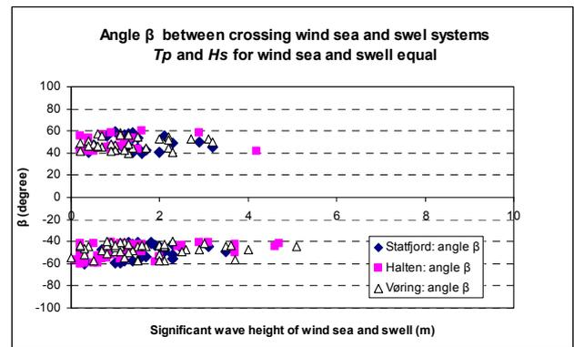
Figure 5. The angle between wind sea and swell having almost the same spectral period and significant wave height as a function of  $H_{sw}$  ( $H_{ss}$ ). The Statfjord, Halten and Vøring locations.
