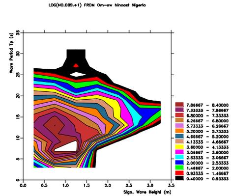
Figure 3. Contour plot of long term significant wave height  $H_{m0}$  and spectral peak period  $T_p$  for total sea; a) data from NWS Australia (1994-2005), Nigeria swell data (1985-1999).
