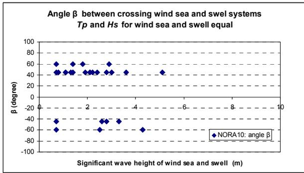
Figure 4. The angle between wind sea and swell having almost the same spectral period and significant wave height as a function of  $H_{sw}$  ( $H_{ss}$ ). NORA10 data, the North Atlantic location.
