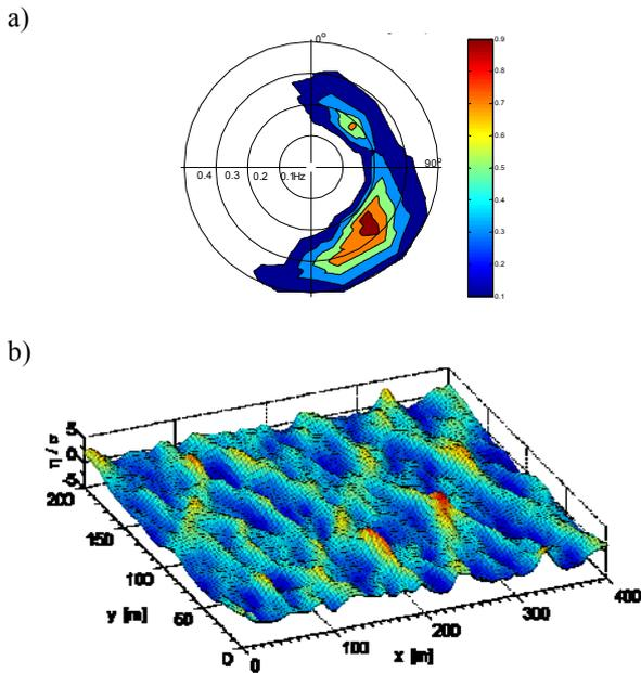
Figure 1. An example of the wave directional spectrum and sea surface when two wave systems are present. Numerical simulations were performed by HOSM.
