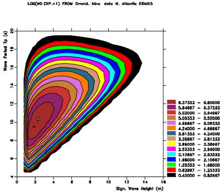
Figure 2. Contour plot of long term significant wave height  $H_{m0}$  and spectral peak period  $T_p$  for total sea, fitted model; a) NORA10 (1958-2009), b) ERA-Iterim (1989-2008).
